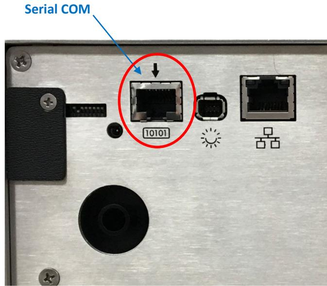
**Figure 4-2 Serial COM Port**
