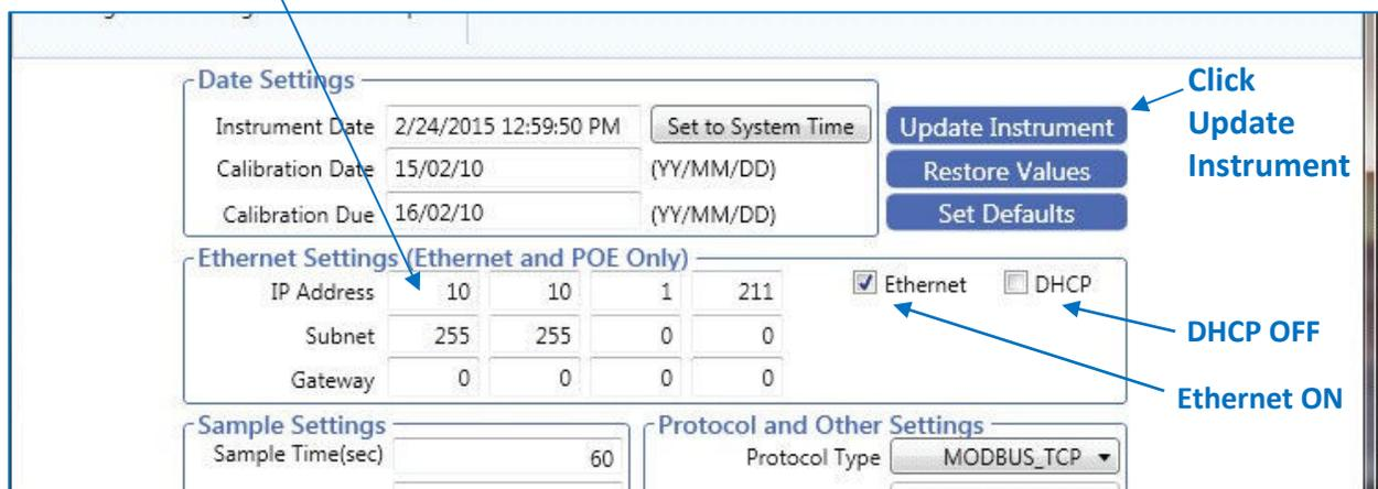
Figure 4-4 Instrument Setup Tool TCP/IP Set Up Screen
