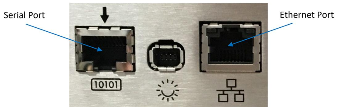
**Figure 7-7 Serial and Ethernet Instrument Connections**
