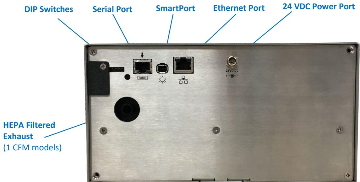
Figure 7-8 ApexRp Connections
