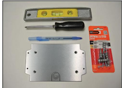
2. If the optional **Wall Bracket** was not ordered, the body of the **ApexRp** can be used as a template to mark the two mounting holes. Make sure the instrument is level then use a pencil to mark the center of the mounting holes. The distance between the holes should be 5.75". Proceed to step 4.
