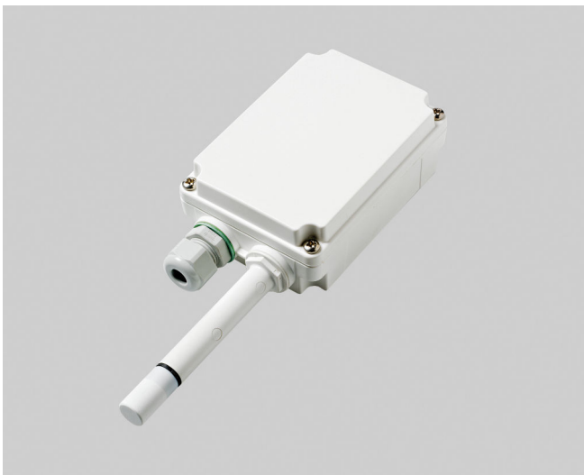
HMW110/112 wall-mount RH+T transmitters with IP65 rating. Model options also include a display version and the TMW110 temperature transmitter. HMW110 and TMW110 transmitters can be ordered either with a cable gland and screw terminal wiring, or with an M12 connector.
