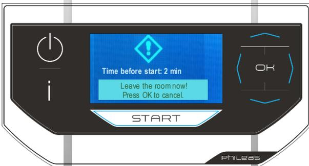
The selected program has a time delay of 1 min, so you have this time to stop the equipment or leave the airlock.
