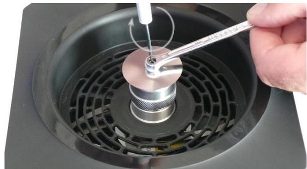
Carrefully remove the disc.
