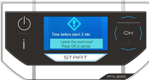
The selected program has a time delay of 1 min, so you have this time to leave locked room.
