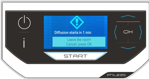
The selected program includes a delay time of 1 min. You have this time to make sure the disinfectant container is full and to leave the room.
