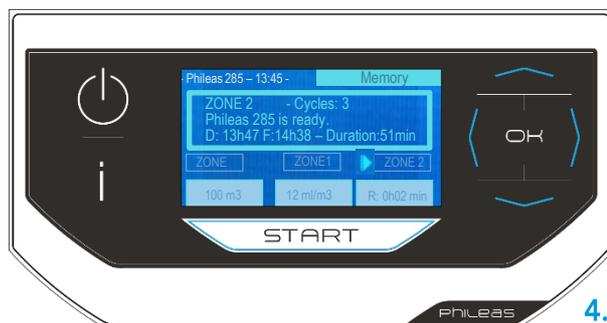
In this example (4.), the arrow points ZONE 2, with different diffusion parameters (volume, dosage, cycles, total duration, delay time).
