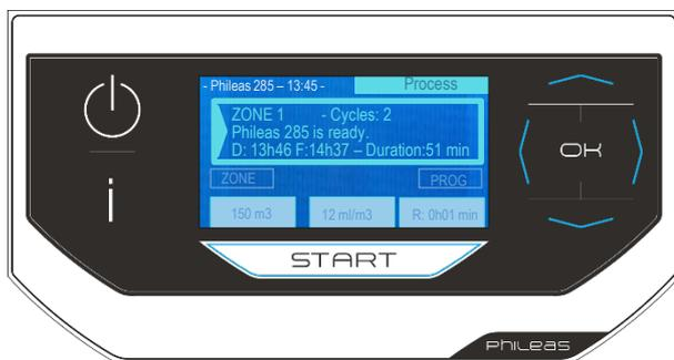
The following screen is the *Process* mode. It shows the parameters of the last diffusion program used.
