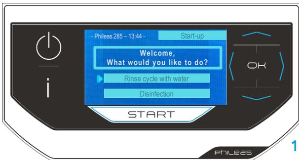
Press **ok** to *Confirm the diffusion* of the rinse cycle or the water test and confirm **GO !** By pressing ok again.
