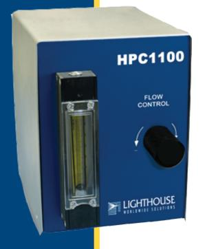
ESIGNED using the latest technology in high-pressure gas components, the High Pressure Controller 1100 allows attachment of a Lighthouse 0.1 µm particle counter to high pressure (30-150 psi) inert gas systems to provide monitoring capability for process gas contamination.
