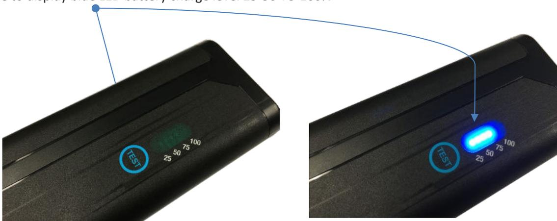
**Note:** The ApexZ Smart Batteries have a power-saving function where they will go into a hibernation mode after not being used for a period of a few weeks. While in this mode pressing the Test button will not show any charge present on the battery, and the battery will not power the unit. To “wake” the battery, power must be applied to it, such as being inserted into an ApexZ unit that has DC power applied.
