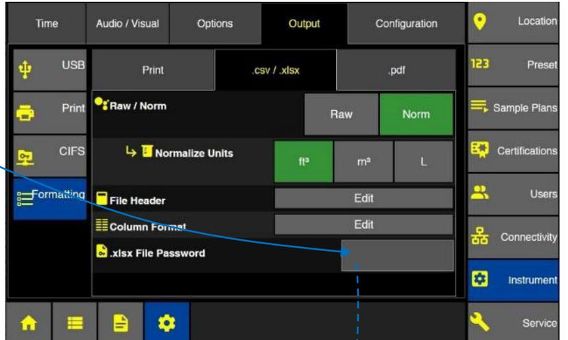
Use the keyboard to enter the desired password, and verify the password by entering it a second time. A maximum of 16 characters can be entered. Press the green Apply button to verify the entries.
