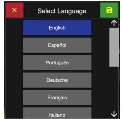
**Warning:** Changing the instrument language will update the instrument firmware and the printer. It will take 1-2 minutes for the update to complete. During this time make sure the ApexZ instrument has at least 50% battery life remaining or connected to the AC adapter and do not turn off the instrument while updating. Failure to follow these instructions could cause the printer to become damaged and unusable.
