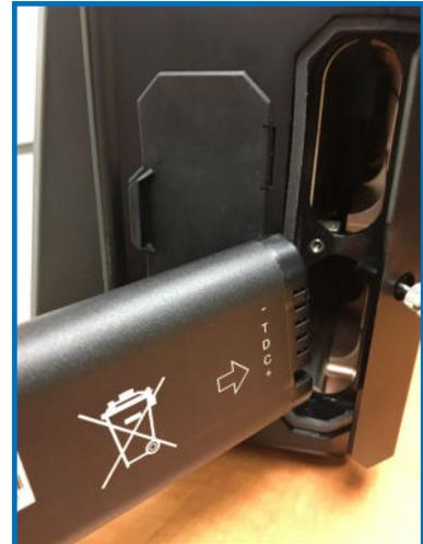
Insert **battery 2** into the upper battery bay. You will feel a slight pressure and clicking as the battery seats down fully in the battery bay.
