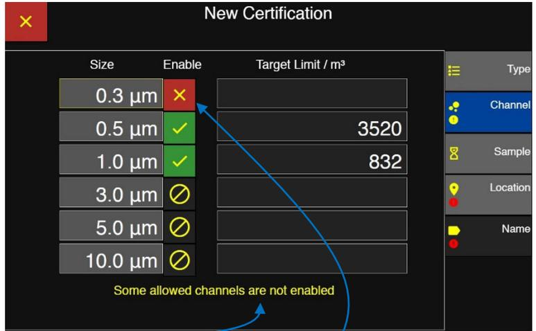
In this example the 0.3 µm size particle channel is an allowed channel but it was disabled. Target Limits are not shown for disabled channels.
