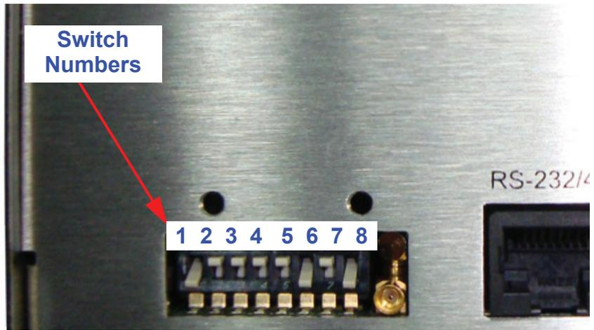
Figure 4-2 Panel Removed, Switches Exposed
