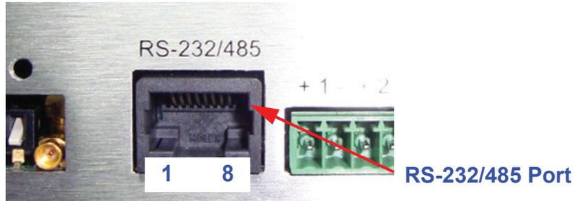
Figure 4-3 The Programming Port, Showing Pin Numbers
