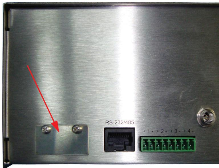
**Figure 4-1 Panel Covering the DIP Switches**
