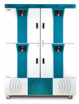
JSMI-04CP 125 Liter Four Chamber Incubator provides multiple chambers in a compact unit share less footprint. Temperature of each chamber can be controlled independently. Equipped with programmable Controller provides 10 Steps of temperature programming control or constant temperature. Temperature range from +0 °C to +70 °C. Suitable for incubation of microorganism needs temperature and light at the same time and various test for food and packaging test on QA / QC labs.
