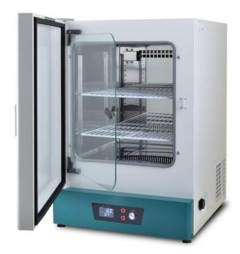
JSBI-100CP Programmable Tabletop Refrigerated Incubator provides 10 Steps of temperature programming or constant temperature operation range from  $+0^{\circ}$ C to  $+70^{\circ}$ C for more versatile use. It gives excellent performance for incubation of microorganisms, BOD (Biological Oxygen Demand) Test and various QA / QC Tests.
