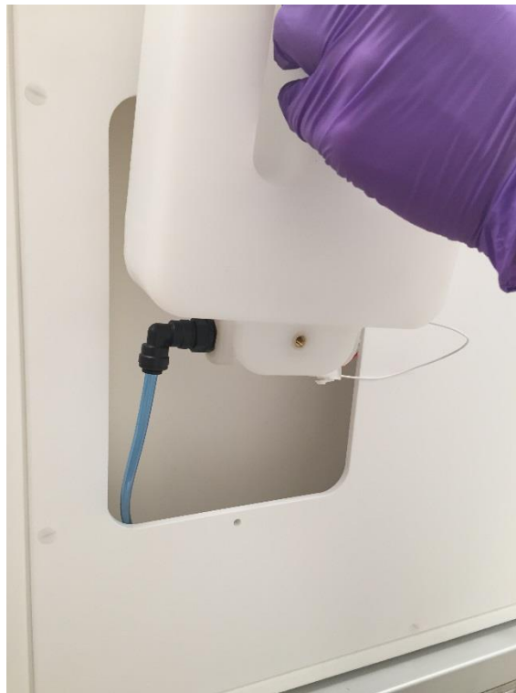
Figure 30: Water Tank bottom lifted out
