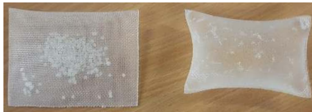
Figure 22: Aquasorb Sachets - Empty and Charged
