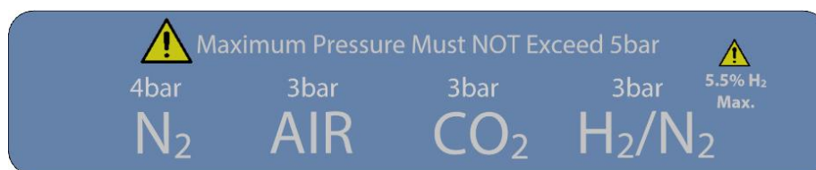
Figure 2: Gas Connection Graphic
