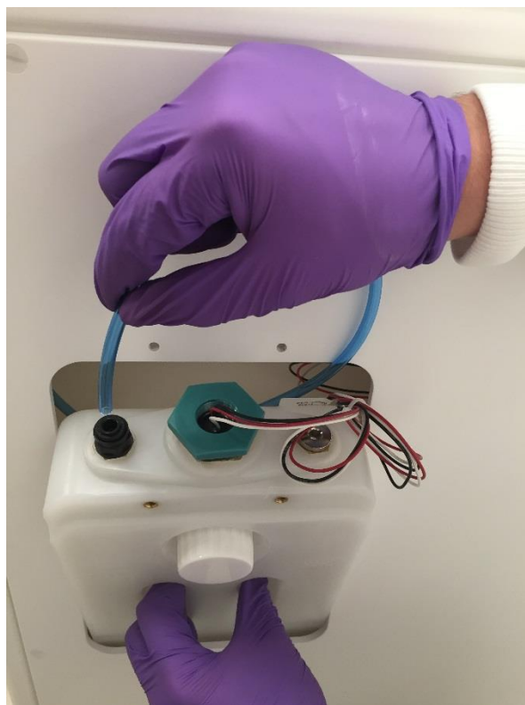
Figure 28: Water Tank top tube removal
