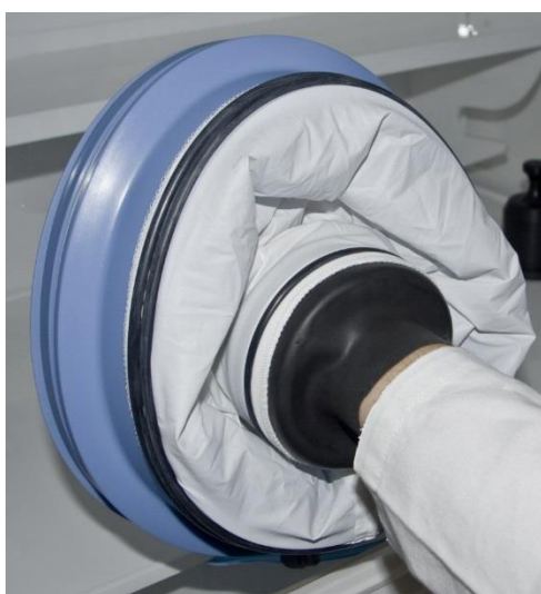
Figure 15: Ezee-Sleeve before vacuum
