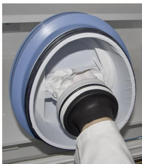
Figure 16: Ezee-Sleeve after vacuum
