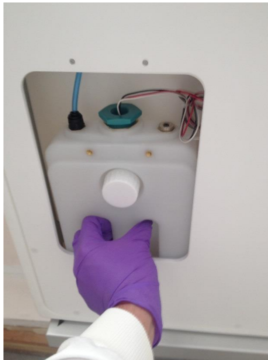
Figure 26: Water Tank lowered for removal
