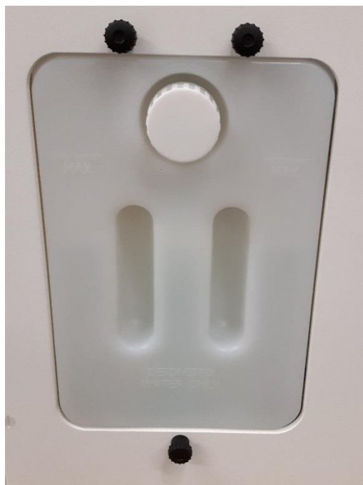
Figure 24: Humidity System Water Tank
