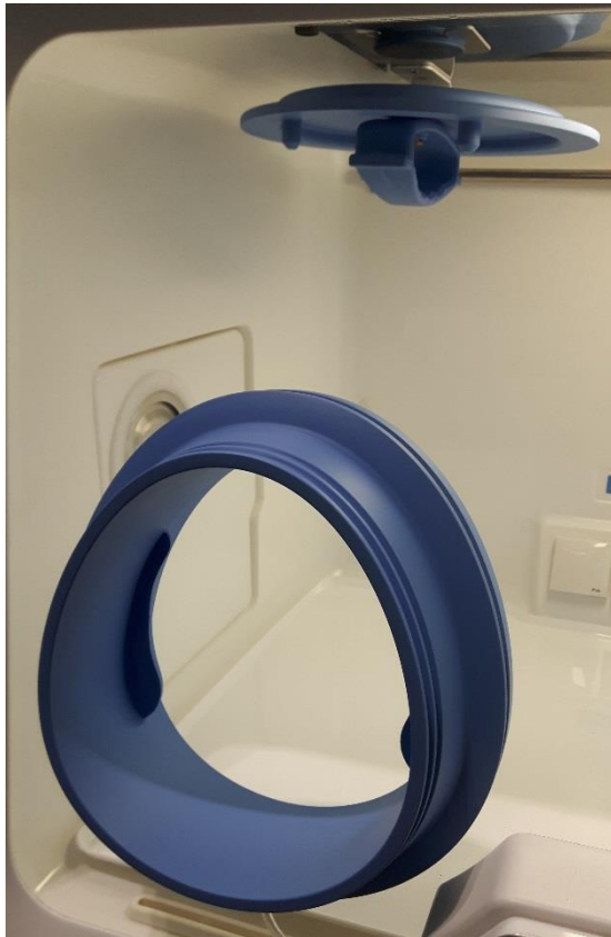
Figure 19: Glove port cap storage location inside workstation
