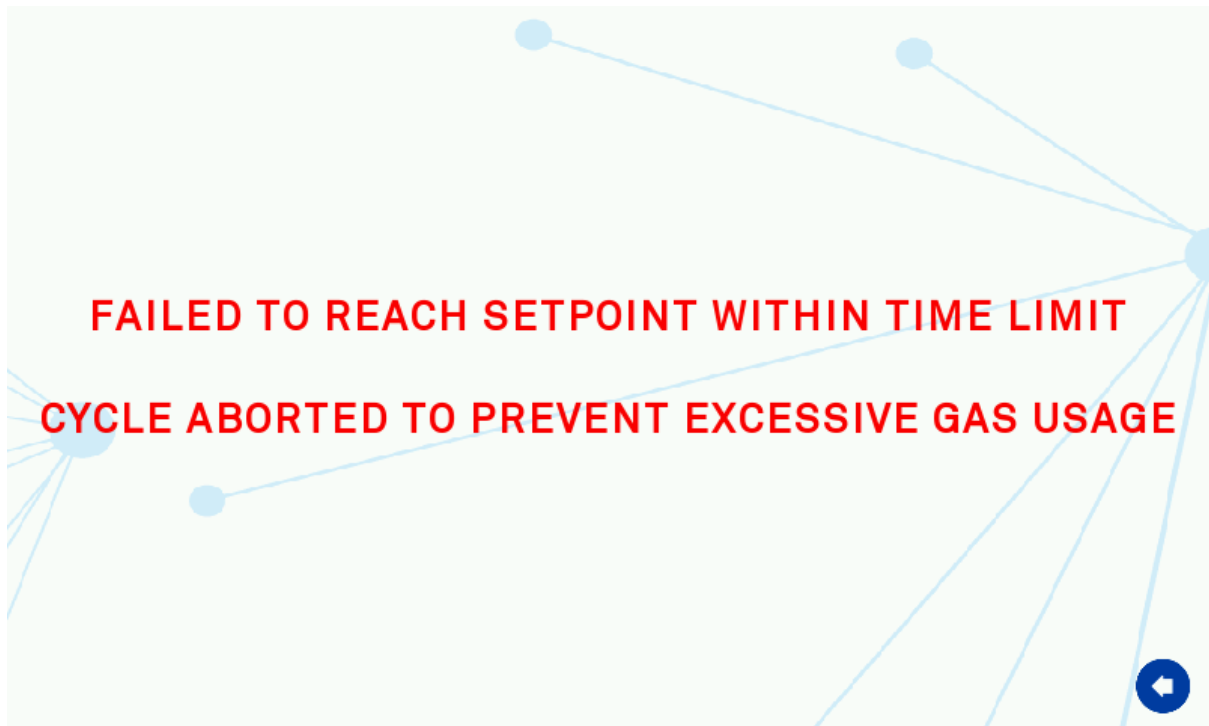
Screen 23: Gas Mix Time Limit Warning Screen
