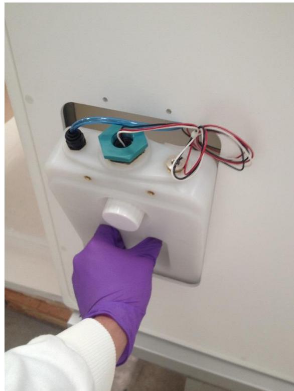
Figure 25: Water Tank tilted forward partially removed
