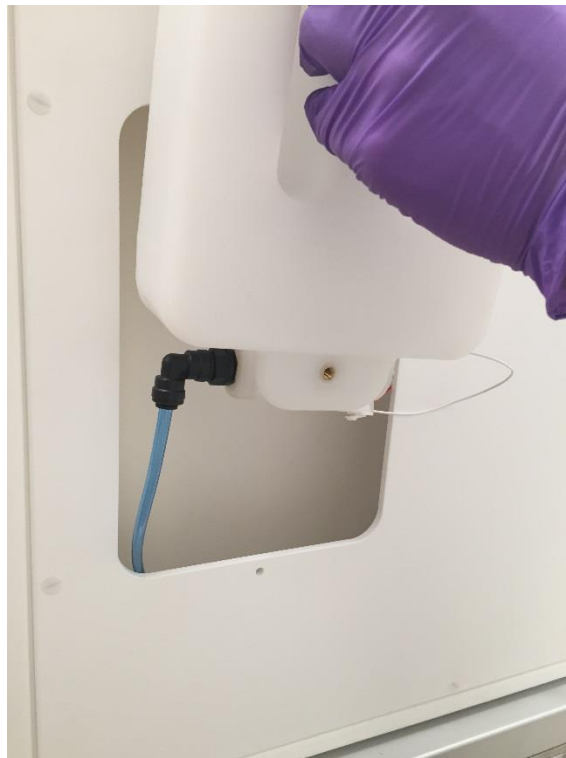
Figure 28: Water Tank bottom lifted out
