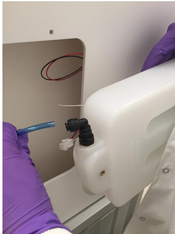
Figure 29: Water Tank bottom tube disconnection
