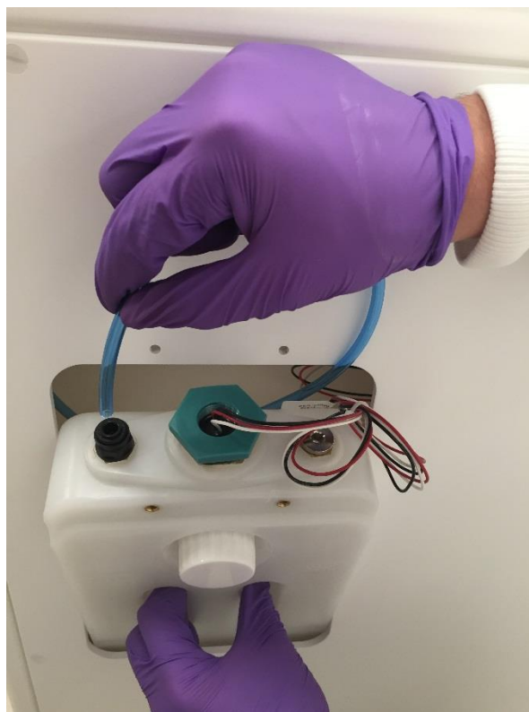
Figure 26: Water Tank top tube removal
