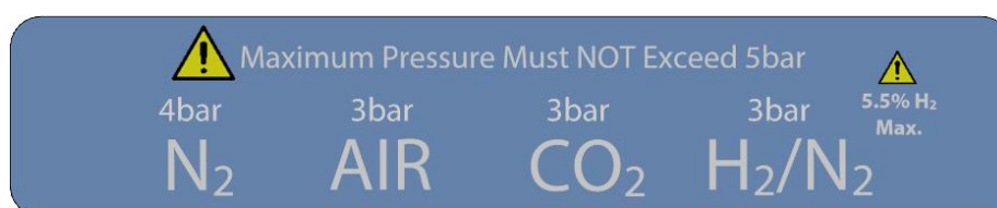
Figure 2: Gas Connection Graphic
