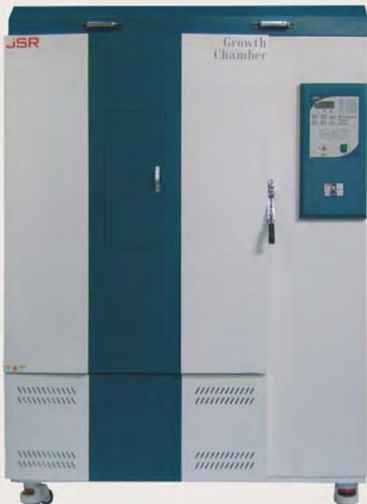
JSGC-Series Top Illumination Plant Growth Chamber provides reliable controlled climatic condition of temperature, humidity, lighting and CO<sub>2</sub> concentration
