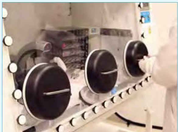
Removable front cover with triple glove ports makes the SCI-tive easy to use.
