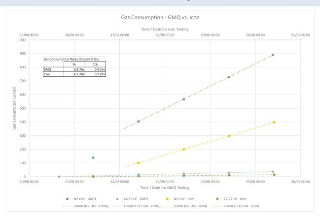
**I-CO<sub>2</sub>N<sub>2</sub>IC Gas Consumption Test.** The results of a steady-state test (InvivO<sub>2</sub> 400 set to 0.1% O<sub>2</sub> and 0.5% CO<sub>2</sub>). ICO<sub>2</sub>N<sub>2</sub>IC used 296 L of N<sub>2</sub> over the test period, a reduction of 40% over the previous technology.
